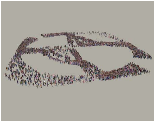
Fig. 7.13. Conditions under which the tests have been achieved: five human templates, steering and animation enabled, no shadows, no accessories, no collision avoidance.
